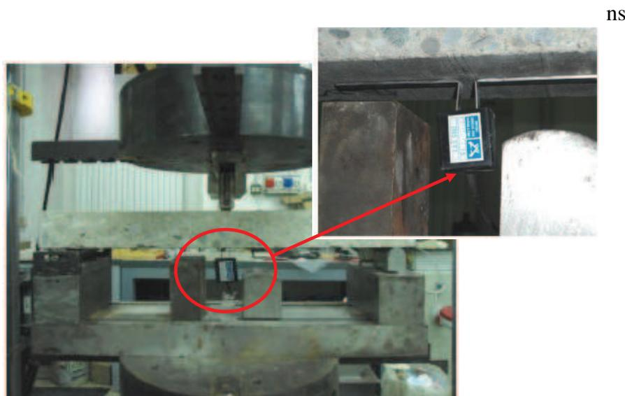
Figure 4: 3-point bending test set-up for specimen pre-cracking (beam span = 450 mm).
