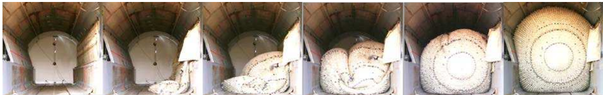
Figure 3: Sequence of initial unrolling and inflation captured during full-scale tests ( Barbero et al. 2013a ; Sosa et al. 2014a ).
