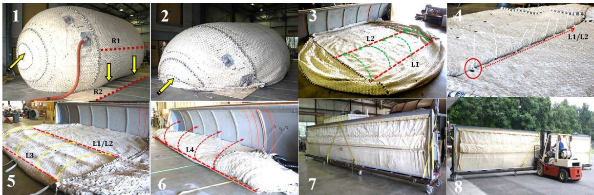
Figure 1: Sequence of folding and packing implemented experimentally (Barbero et al. 2013a; Sosa et al. 2014a).
