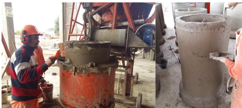
Figure 1: a) moulding and vibrating process b) surface finishing
