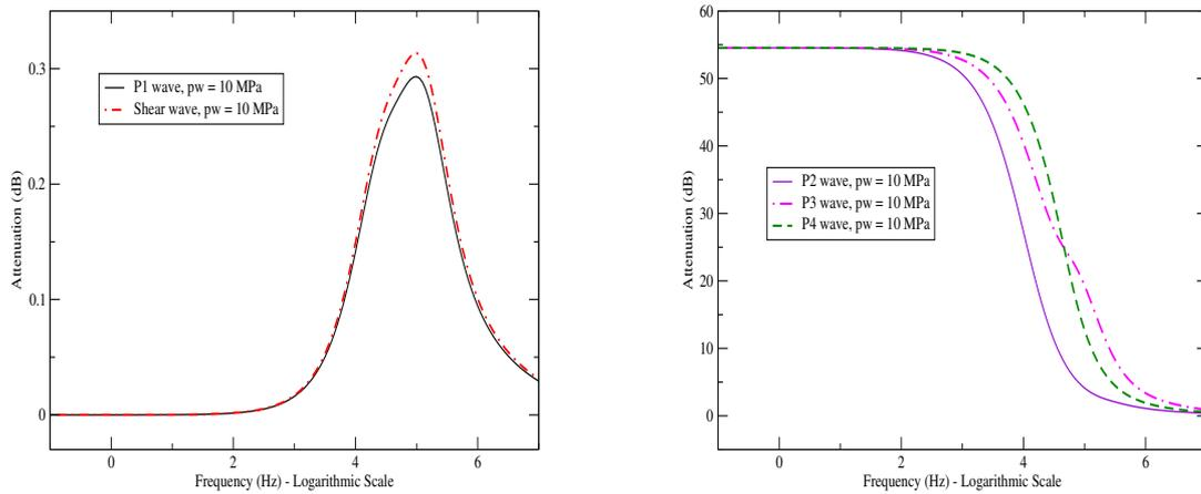
Figure 7: P1, Shear (left) and P2, P3, P4 (right) wave attenuation (dB) as function of frequency at  $S_w = 0.25$ ,  $S_g = 0.1$  and  $\bar{p}_w = 10$  MPa
