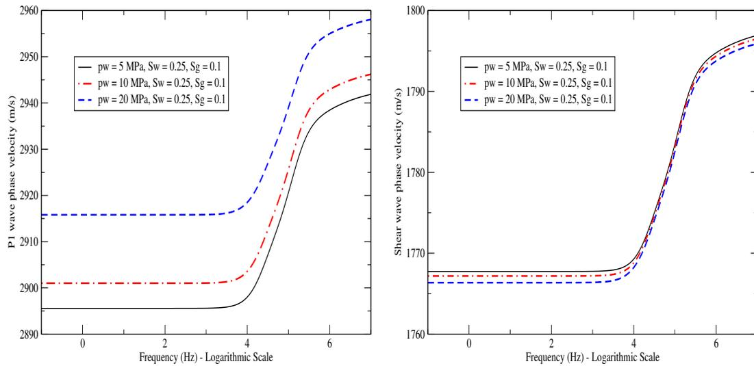
Figure 4: P1 (left) and Shear (right) wave phase velocity as function of frequency at  $S_w = 0.25$ ,  $S_g = 0.1$  and  $\bar{p}_w = 5, 10$  and  $20$  MPa
