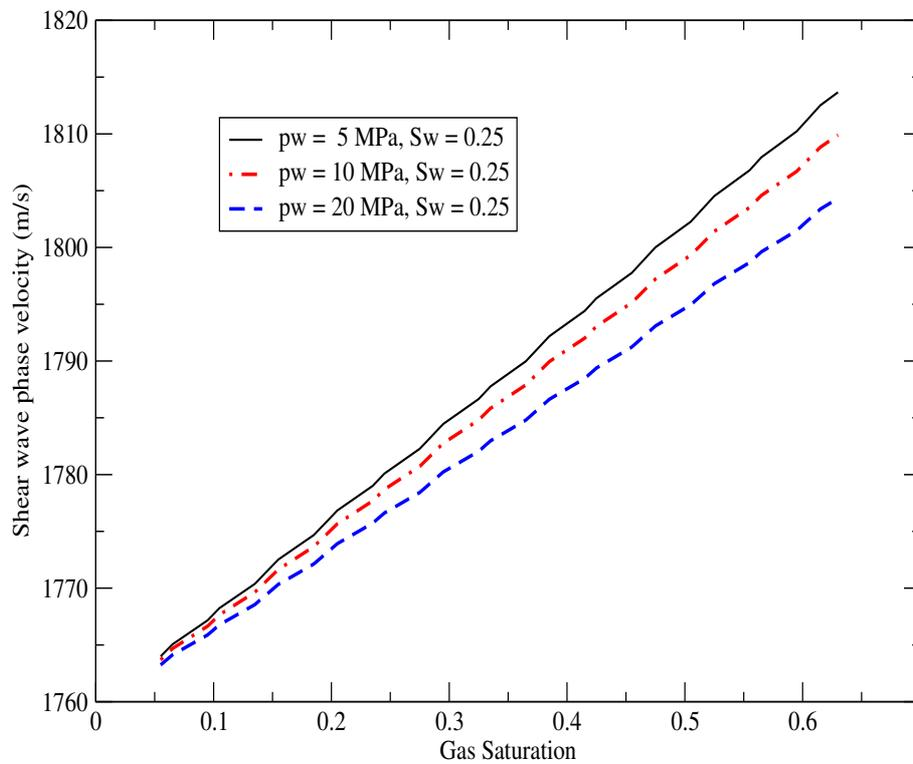
Figure 3: Shear wave phase velocity as function of gas saturation at  $S_w = 0.25$  and  $\bar{p}_w = 5, 10$  and 20 MPa.
