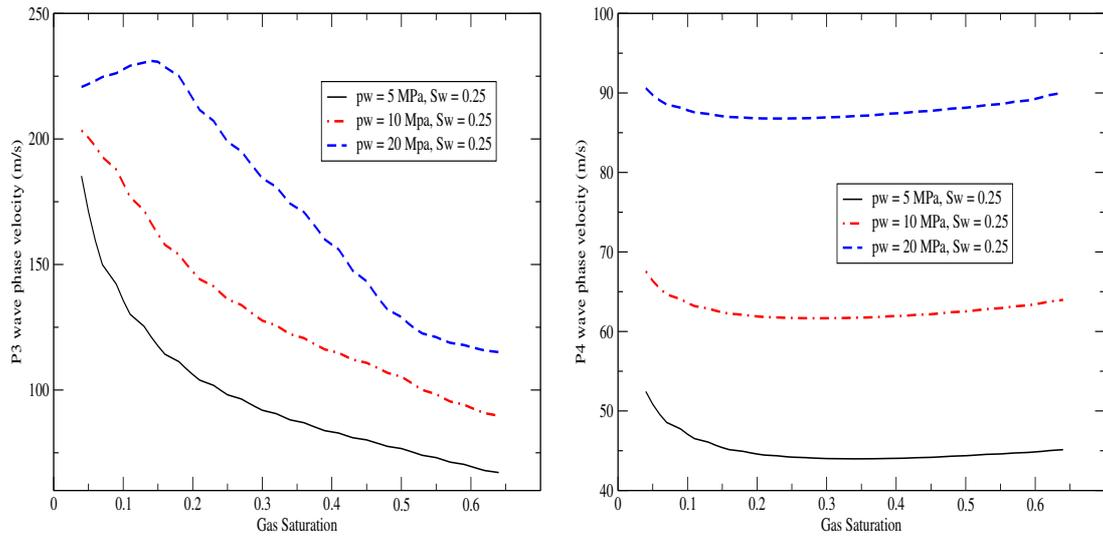
Figure 2: P3 (left) and P4 (right) wave phase velocity as function of gas saturation at  $S_w = 0.25$  and  $\bar{p}_w = 5, 10$  and 20 MPa
