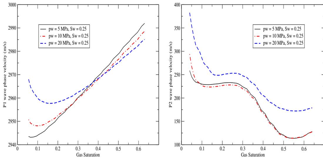
Figure 1: P1 (left) and P2 (right) wave phase velocity as function of gas saturation at  $S_w = 0.25$  and  $\bar{p}_w = 5, 10$  and  $20$  MPa
