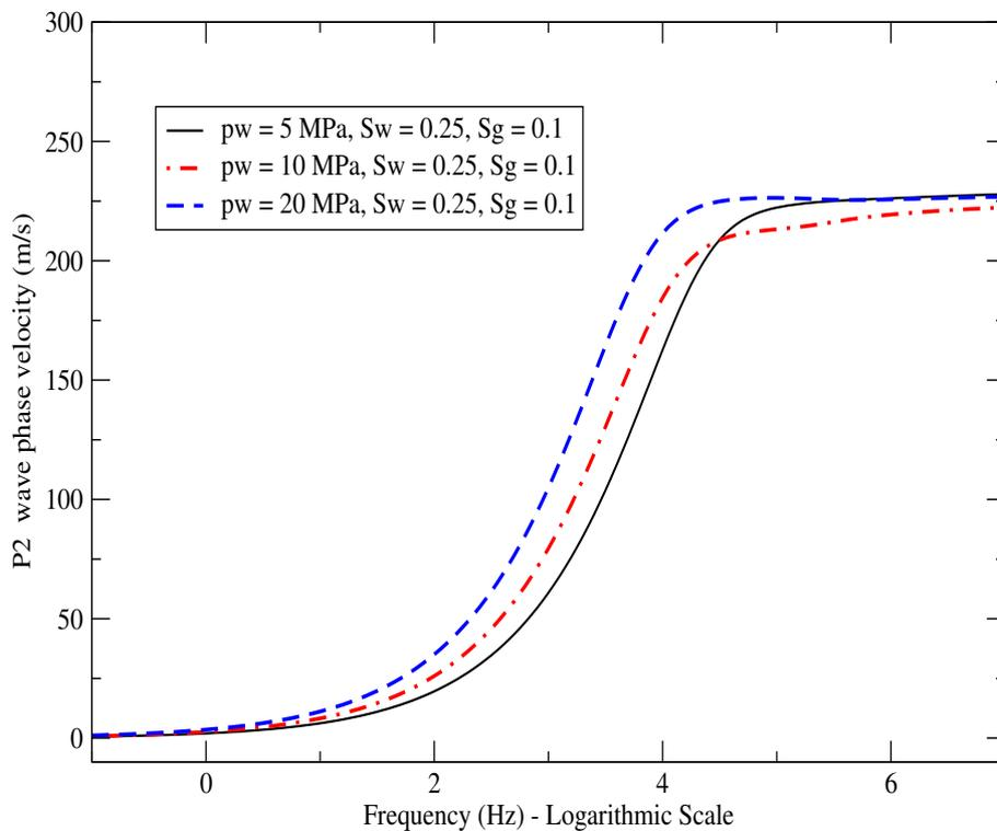
Figure 5: P2 wave phase velocity as function of frequency at  $S_w = 0.25$ ,  $S_g = 0.1$  and  $\bar{p}_w = 5, 10$  and  $20$  MPa
