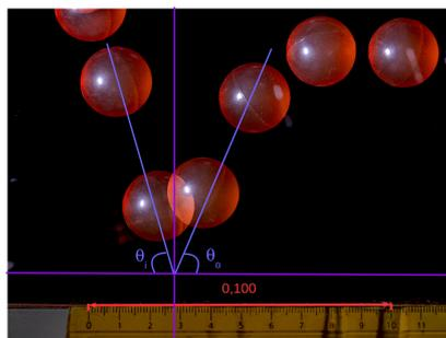
Figure 2: Superposition of frames extracted from the Tracker Software (Brown, 2015). The axes origin is the ball center of mass.
