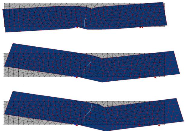
(d) Crack propagation by the Generalized Finite Element Method (Silva, 2016).
