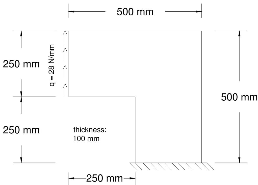
Figure 5: L-Shaped panel - Structural scheme.
