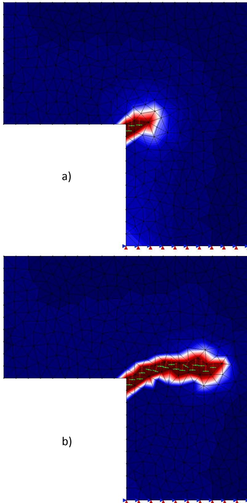
Figure 6: L-Shaped panel - a) Localization analysis at early step, b) Localization analysis at late step
