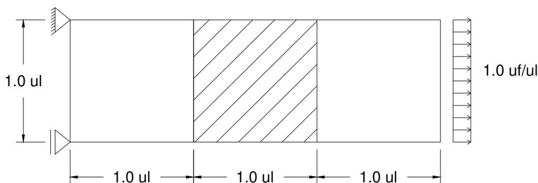
Figure 2: Uniaxial tensile test - Structural scheme.
