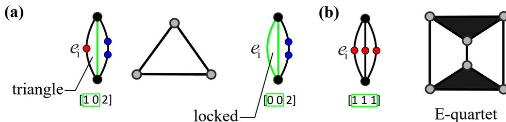
Figure 2: One- and two-loop locked 1-DOF kinematic chains. Triangles can be identified from the assignment vector of binary chains(a) whereas E-quartets can be identified from assignment vectors: more complex E-quartets can appear as subgraphs and require the listing of paths of length 2 between two higher-links. Rigid subchains with 3 or more loops can be included in the tests presented in this paper.
