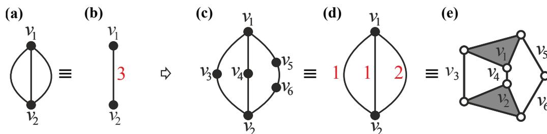
Figure 1: A contracted graph represented by a multigraph (a) or by labeled simple graph (b) where labels indicated edge multiplicity. The contracted graph is used as a basis to assign binary strings (c) and (d) to form a kinematic chain (e)
