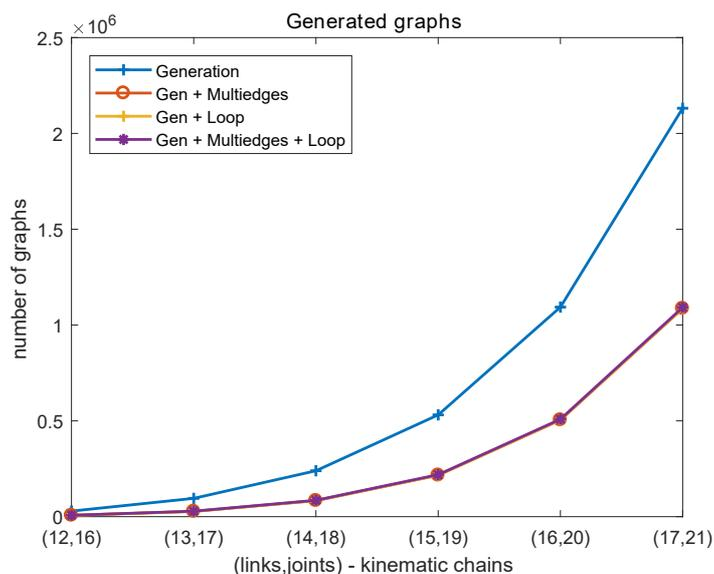
Figure 5: Number of feasible graphs enumerated. There is no appreciated difference in the graphs. However, the *Multiedges* experiment is not correct.
