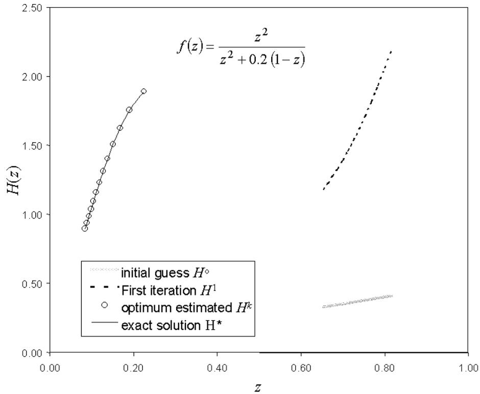
Figure 3: Estimation of the derivative of the fractional flow curve for example 2
