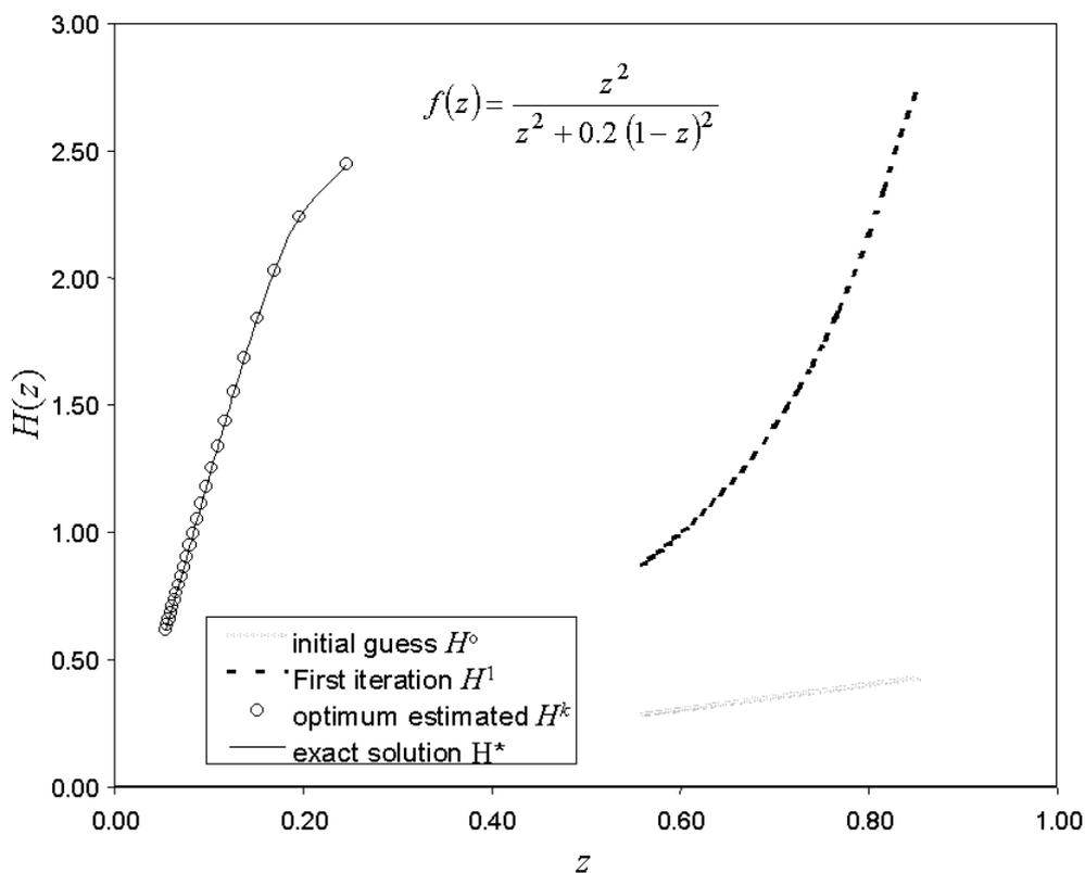
Figure 1: Estimation of the derivative of the fractional flow curve for example 1
