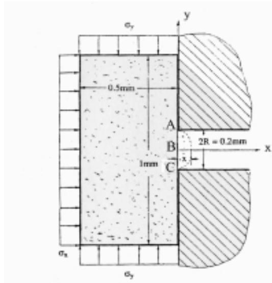
**Figure 1.** Bone tissue structure subject to tensions  $\sigma_x$  y  $\sigma_y$ , that may grow into a slot.
