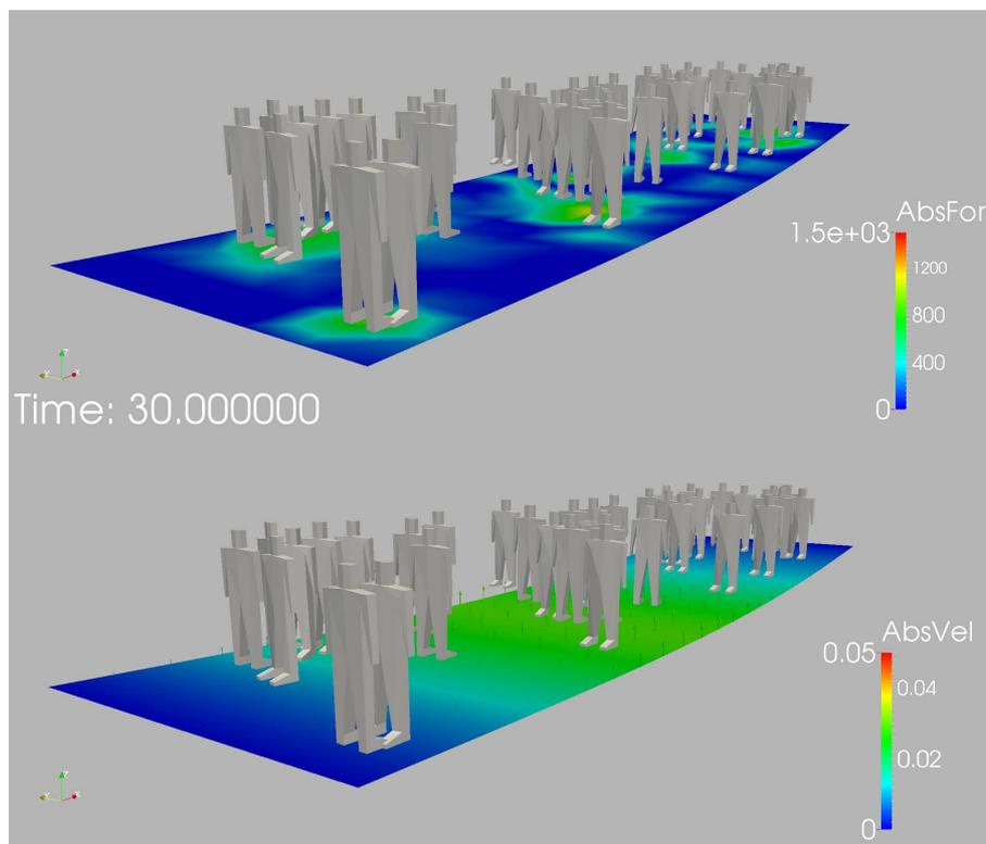
Figure 2a Force and Velocities of the Structure at T=30 sec
