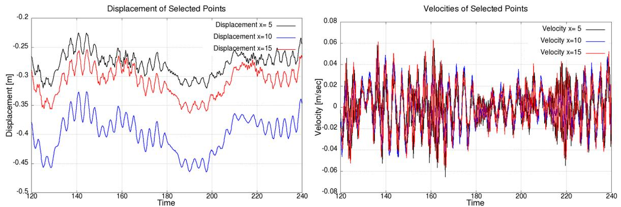
Figure 2d,e Displacements and Velocities of Three Selected Points on the Bridge
