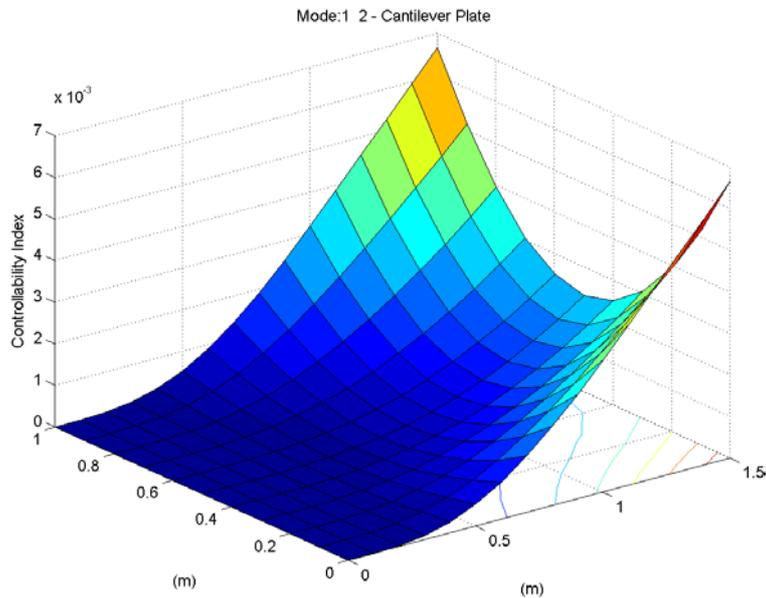
Figure 3: Controllability Index - singular values between 1<sup>o</sup> and 2<sup>o</sup> mode.
