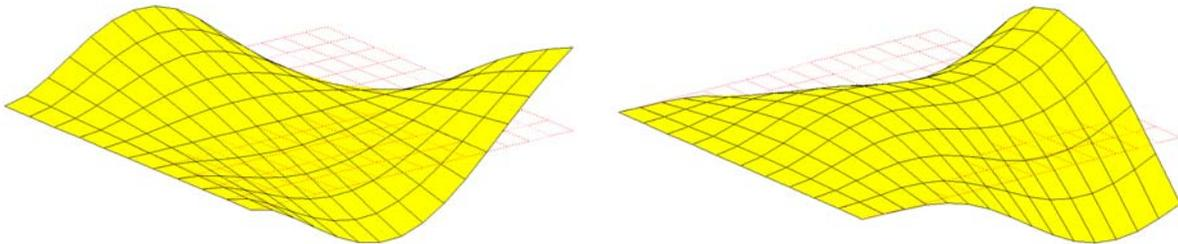
Figure 8: Cantilever in 4<sup>o</sup> and 5<sup>o</sup> mode shape.
