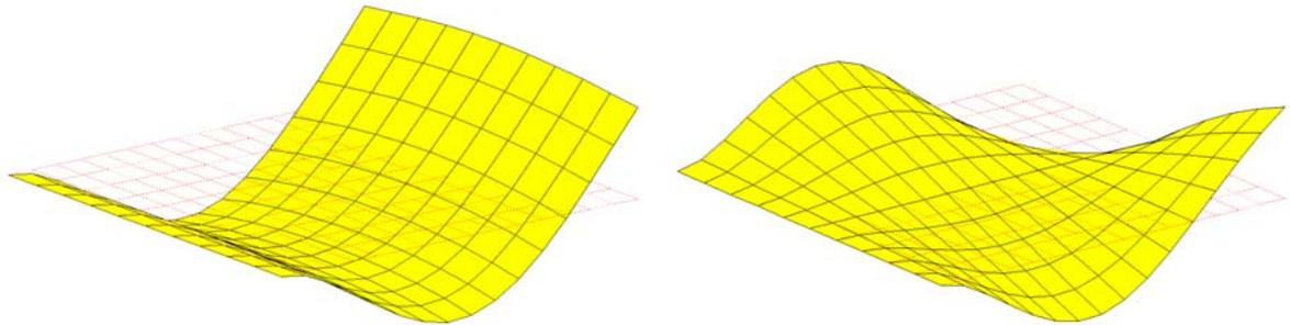
Figure 6: Cantilever in 3<sup>o</sup> and 4<sup>o</sup> mode shape.
