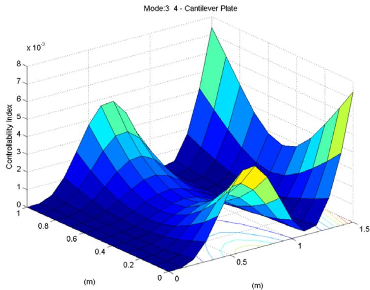
Figure 7: Controllability Index - singular values between 3<sup>o</sup> and 4<sup>o</sup> mode.
