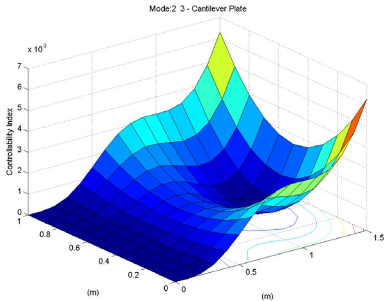
Figure 5: Controllability Index - singular values between 2<sup>o</sup> and 3<sup>o</sup> mode.
