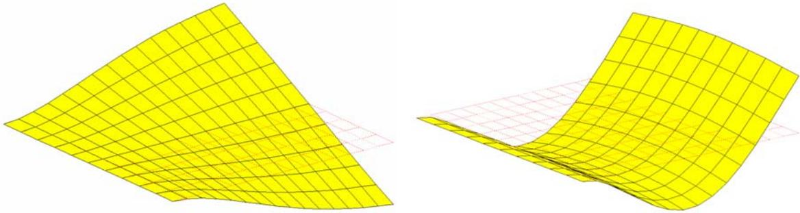
Figure 4: Cantilever in 2<sup>o</sup> and 3<sup>o</sup> mode shape.
