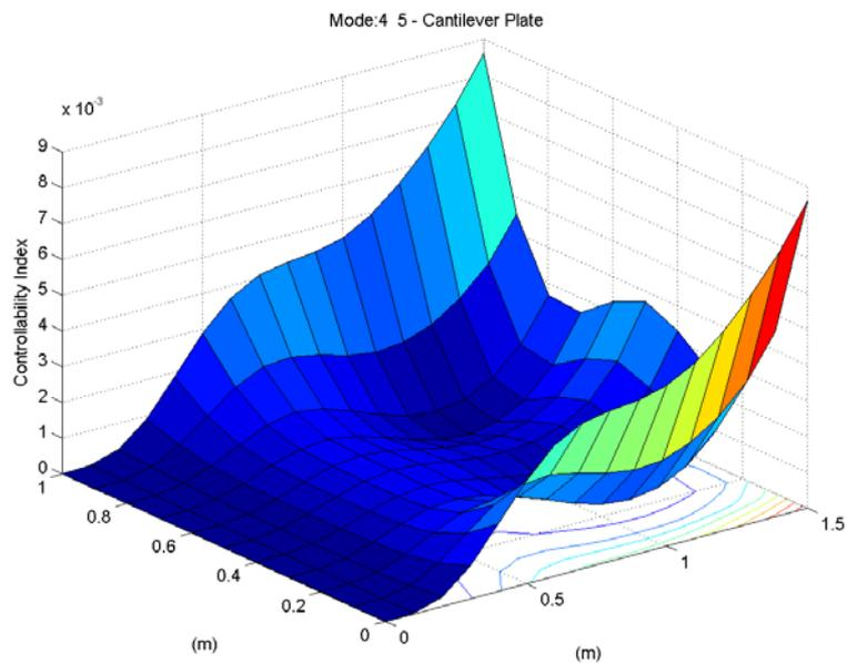
Figure 9: Controllability Index - singular values between 4<sup>o</sup> and 5<sup>o</sup> mode.
