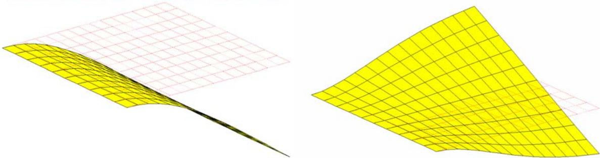
Figure 2: Cantilever in 1<sup>o</sup> and 2<sup>o</sup> mode shape.
