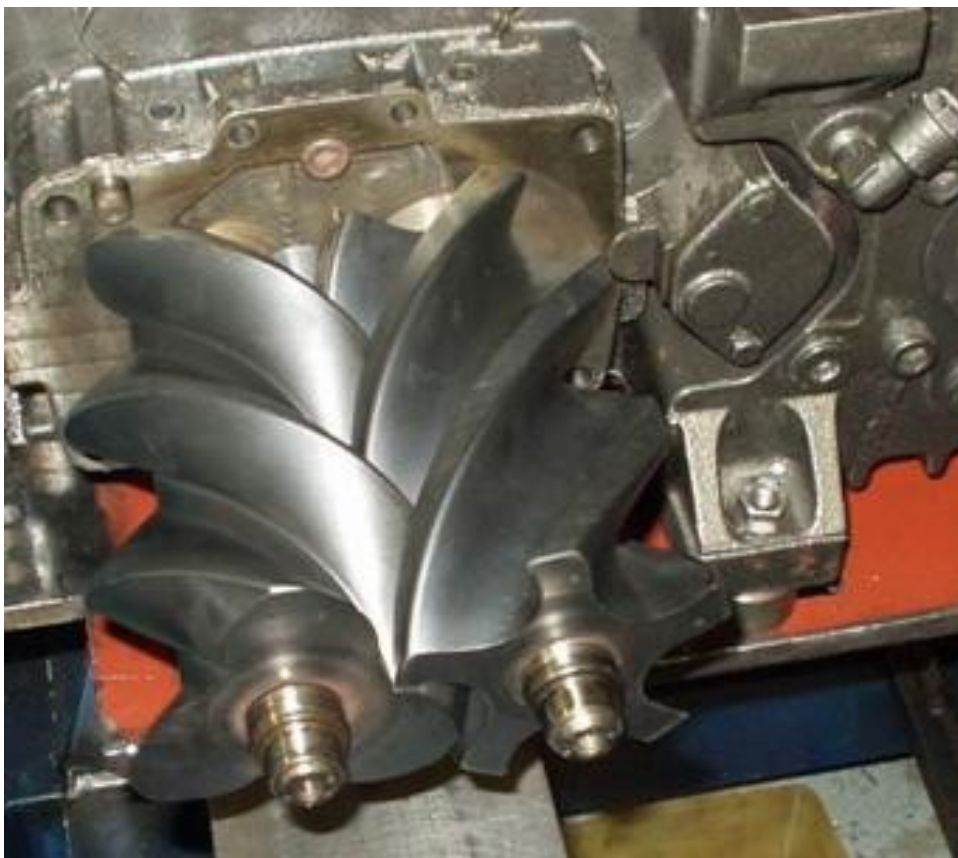
Figure 7: Compressor rotors, housing removed
