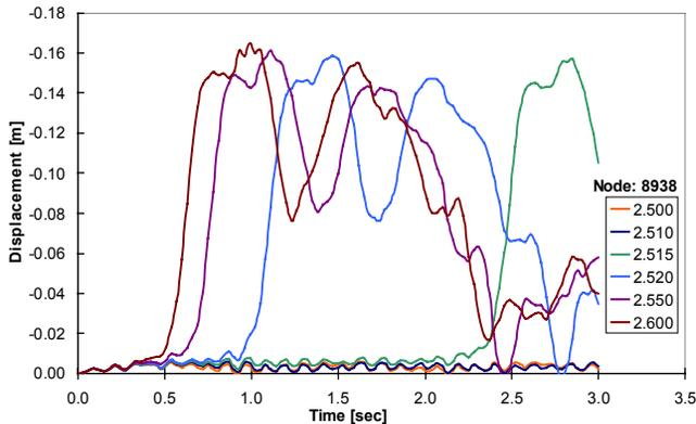
Figure 4. Nonlinear dynamic response for 3 sec wind gust assumed constant. Each curve is for different pressure amplitude. Instability occurs for  $\lambda = 2.515$ .
