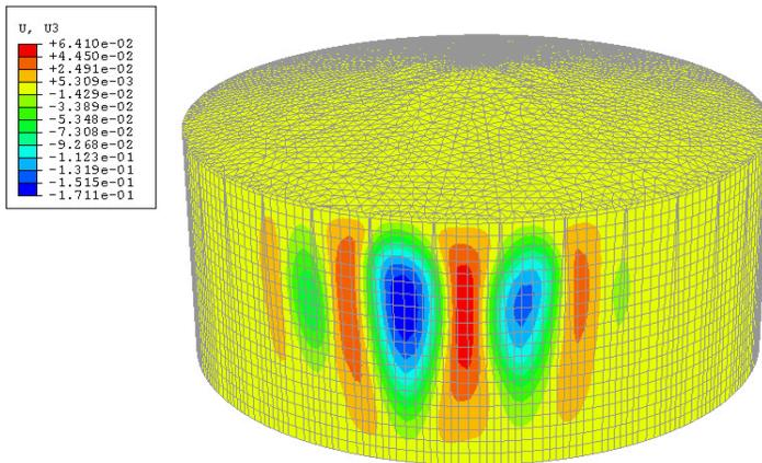
Figure 6. Nonlinear dynamic analysis, deflected pattern for  $\lambda = 2.55$ , at time  $t=3$  sec.
