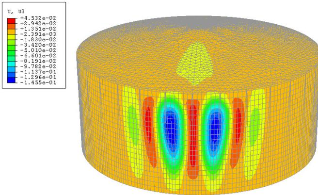
Figure 5. Nonlinear dynamic analysis, deflected pattern for  $\lambda = 2.515$ , at time  $t=2.55$  sec.
