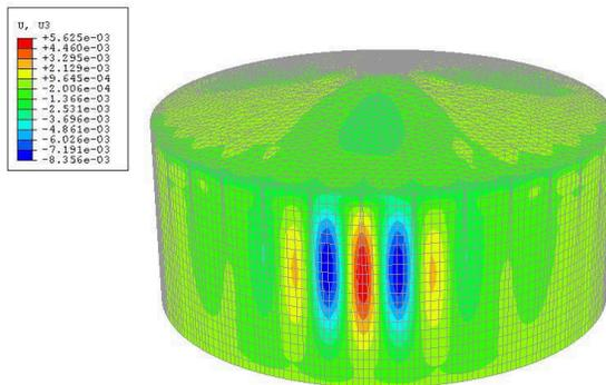
Figure 8. Static nonlinear analysis, deflected shape for  $\lambda = 2.55$ .
