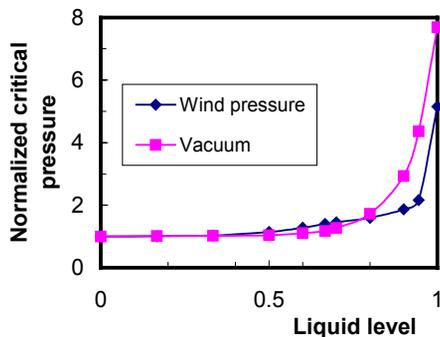
Figure 1. Influence of liquid level on the critical pressures of tanks. The results for wind pressure are for an open-top tank<sup>10</sup>, while the results for vacuum<sup>22</sup> correspond to a simply-supported condition at the top.
