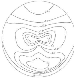
Figure 3. Pressure distribution assumed on the roof of the tank (after MacDonald *et al.*<sup>25</sup>).
