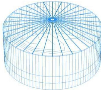
Figure 2. Model of the tank with fixed roof and rafter supports on the roof.
