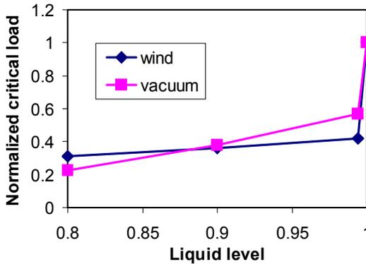
Figure 12. Sensitivity of critical load to a decrease in the liquid level filling the tank. Data as in Figure 1.
