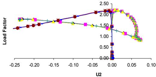
Figure 11. Nonlinear equilibrium paths for an open-top tank with initial load imperfections<sup>20</sup>.
