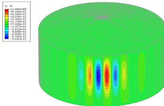
Figure 9. Bifurcation buckling, first mode,  $\lambda = 2.6107$ .
