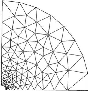
Figure 2. Finite element mesh used in the numerical solution.
