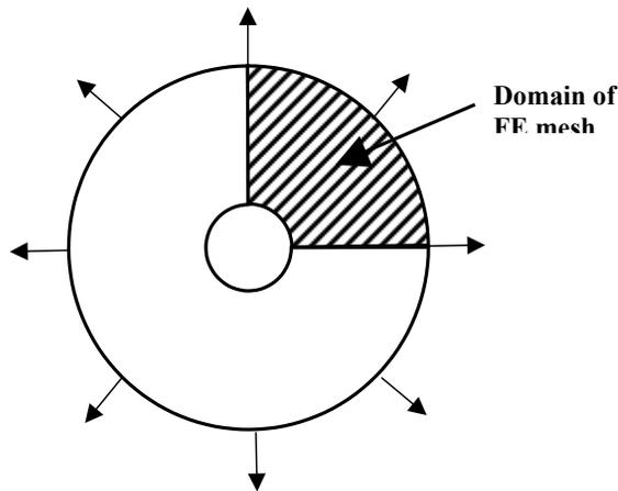
Figure 1. Circular uniform thickness sheet with circular bore subjected to radial pull.
