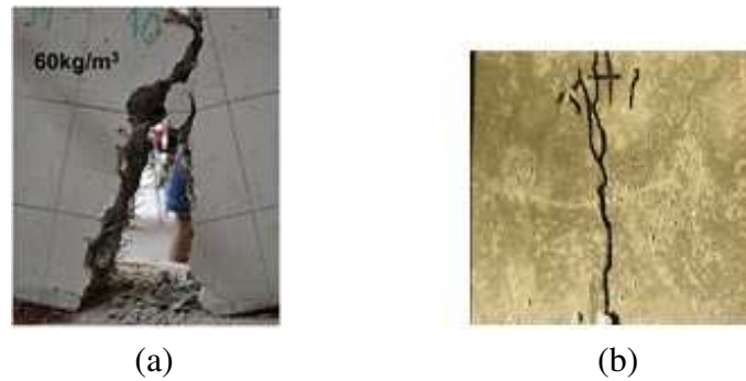
Figure 4: Final view of FRC specimens after the TPB. (a) NSC; (b) HSC.
