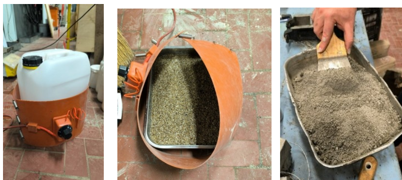
Figure 2: The procedure of preparing mixture of Vermiculite with PCM.
