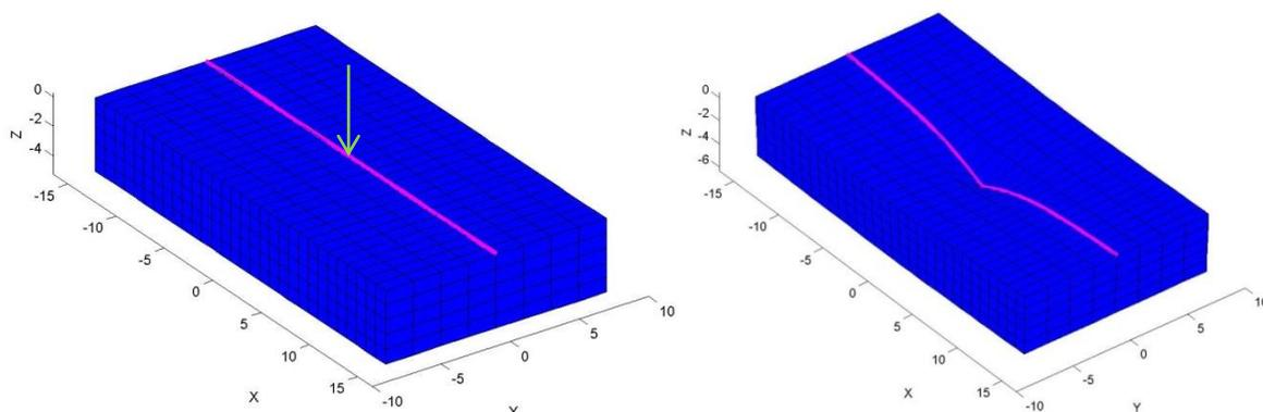
Figure 6. Left figure: Mesh of soil domain supporting beam with moving load/vehicle. Right figure: Stationary deformation for the analyzed case.
