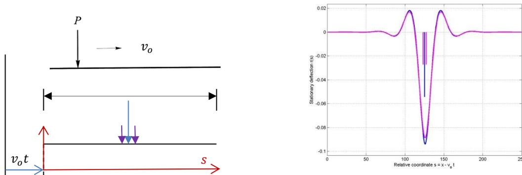
Figure 3. Stationary deformation field  $r_{st}(s)$  for single vertical load (blue lines) and for the same vertical load applied in two nodes (magenta lines)
