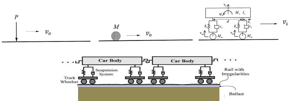
Figure 1. Problems of moving load, mass or vehicle on infinite elastic media.
