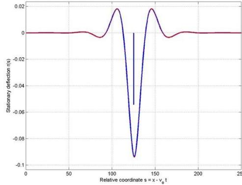
Figure 4. Stationary deformation field  $r_{st}(s)$  for single vertical load (blue line) and for moving mass with the same vertical load (red dots).
