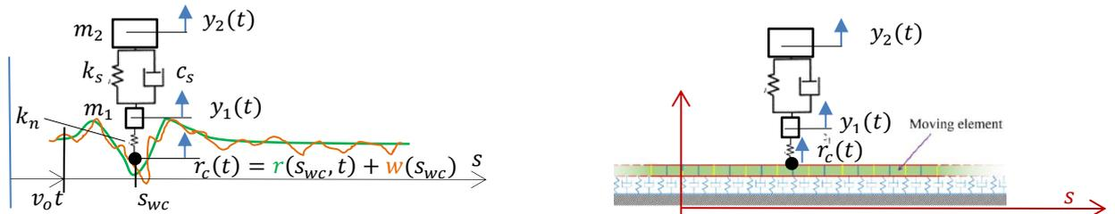
Figure 5. Quarter vehicle model on elastic media with roughness in contact.
