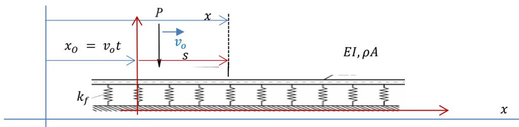
Figure 2. Moving load on a beam on elastic foundation.
